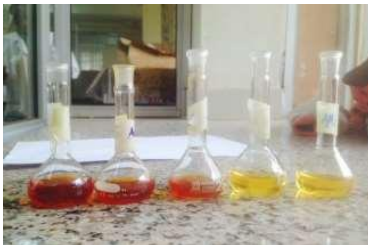
Figure 1. (a) 20ppb which is the highest conc. (b) 5ppb which is the moderate conc. (c) maize sample(1ppb) the lowest conc. (d) water(control) (e) extracting solvent (methanol).
